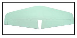
□ 2) Using a modeling knife, carefully remove the covering at mounting slot of horizontal stabilizer (both side of fuselage).
