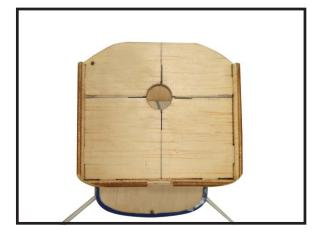
3) Attach the motor to the front of the electric motor box using four 3mm blind nut, four M3x15mm hex head bolts to secure the motor. Please see picture shown.
