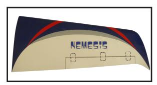
Note: Work the aileron up and down several times to "work in" the hinges and check for proper movement.
