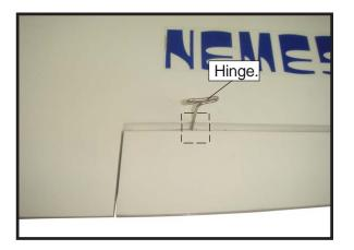
$\Box$  4) Deflect the aileron and completely saturate each hinge with thin C/A glue. The ailerons front surface should lightly contact the wing during this procedure. Ideally, when thehinges are glued in place, a 1/64" gap or less will be maintained throughout the lengh of the aileron to the wing panel hinge line.
