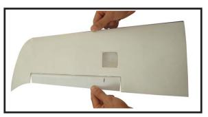
□ 5) Turn the wing panel over and deflect the aileron in the opposite direction from the opposite side. Apply thin C/A glue to each hinge, making sure that the C/A penetrates into both the aileron and wing panel.
