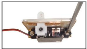
7) Apply 1-2 drops of thin C/A to each of the mounting tabs. Allow the C/A to cure without using accelerator.
