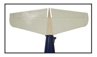
3) Slide the vertical stabilizer back in place. Using a triangle, check to ensure that the vertical stabilizer is aligned 90° to the horizontal stabilizer.
