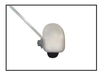
$\Box$  4) A drop of C/A glue on the wheel collar screws will help keep them from coming lose during operation.
