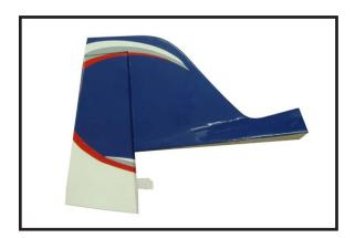
1) Using a modeling knife, remove the covering from over the precut hinge slot cut into the lower rear portion of the tail at the fuselage.
