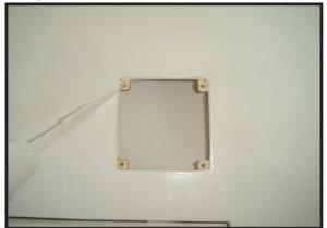
8) A string has been provided in the wing to pull the aileron lead through to the wing root. Remove the string from the wing at the servo location and use the tape to attach it to the servo extension lead. Pull the lead through the wing and remove the string.
